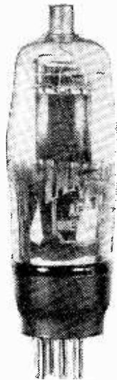
Mazda AC/P4 triode for time-base work.
