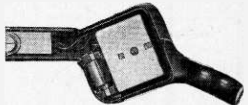
New design of the Telefunken pick-up with permanent needle.
